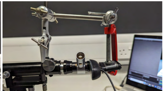
Figure 11: Camera clamped to spectrometer
